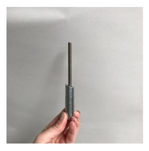
Screw a 4 inch threaded rod into a 1.5" *threaded* spacer. Slide on one Topsy Turvy angled spacer with the angled side facing up.
