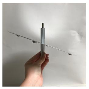
Take another Topsy Turvy angled spacer with the angled side facing down to "sandwich" the plate. Slide a 1.5 inch *non threaded* spacer onto the rod.
